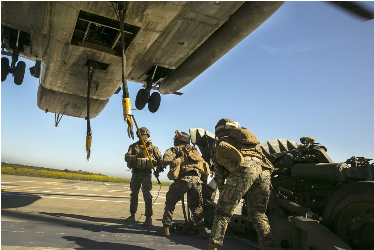
A Marine, left, uses a static discharge wand to discharge excess static electricity before attaching an M777 howitzer to a CH-53E Super Stallion helicopter during integrated slingload training at Marine Corps Base Camp Pendleton, California, April 12, 2017.
